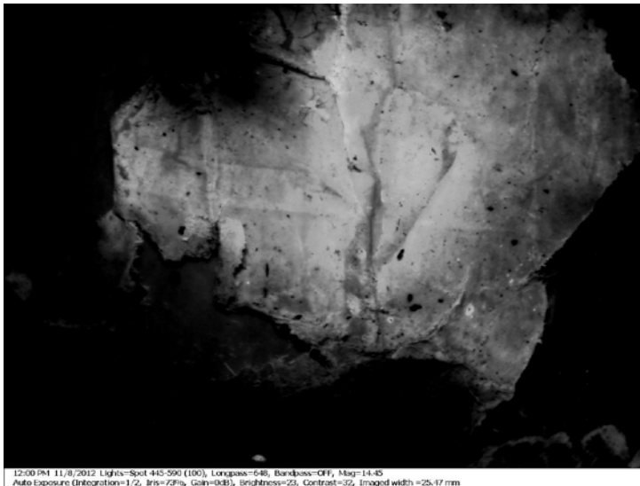
Figure 14 — Image of fragment F1 magnified 15x and obtained with green light (bandpass: 445-590 nm and longpass: 648 nm).
