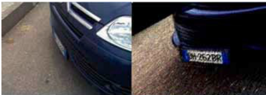
Figure 8: Example of Rectification. It can be appreciated how, in case of planar surfaces, the perspective transformation highlights the information relative to the car license plate.
